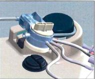
Place the pump loop tubing over the pump rotor. The pump loop will automatically load when the processing cycle is initiated. Seat the platelet cuvette/valve assembly by aligning the platelet cuvette and the valve assembly with the platelet sensor body and the valve assembly driver.
