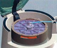
Insert the variable volume separation chamber into the centrifuge adaptor by aligning the notches in the separation chamber plate with the mating feature on the centrifuge adapter.
