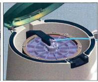
Once aligned, press the separation chamber plate down near the location of the position indicator and turn clockwise until the position indicator snaps into place. • Place the tube leading from the The centrifuge will not rotate if improperly loaded.
