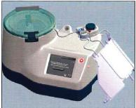
• Press down firmly on the backside • Note: It is essential that the platelet • Hang the three-compartment cuvette/valve assembly seats fully on the machine to obtain proper sensing of blood components.
